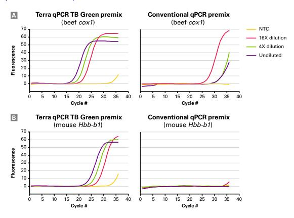
Crude extract amplification comparison between Takra Bio and conventional premixes. Real-time PCR was performed using undiluted, 4X diluted, and 16X diluted crude alkaline-heat extracts of mouse spleen or cow muscle using either Terra qPCR Direct TB Green Premix or a conventional qPCR premix. Data generated by Terra qPCR Direct TB Green Premix corresponded to the theoretical quantities of each gene, while the conventional product was clearly affected by inhibitors present in the crude samples.
