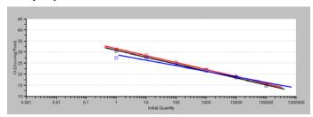
qPCR efficiency was assessed using Cat. # RR420A and other commercially available SYBR master mixes (Companies A, B, and C). Three portions of the ACTB gene were amplified (red: 186 bp; black: 381 bp; blue: 533 bp) from cDNA synthesized using 10 pg to 1 μg of human testes total RNA, and the standard curves were plotted. Takara Bio's TB Green mix outperformed all other mixes.
