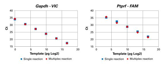
Cat. # RR039A works well in single and multiplex reactions. Real-time PCR was performed on mouse cDNA for Mouse Gapdh or Ptprf using Cat. # RR039A in single and multiplex reactions. Ct values were nearly the same regardless of the type of reaction tested, indicating that the mix works for both experimental setups.
