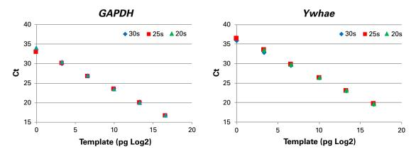
Assessment of shorter extension times. A portion of the *GAPDH* and *Ywhae* genes were amplified by real-time PCR using Cat. # RR390A from cDNA synthesized using 1 pg to 100 ng of total RNA. The standard curves were plotted and reaction efficiency was assessed using various extension times. The same efficiency was obtained with extension times of 20, 25, and 30 seconds.
