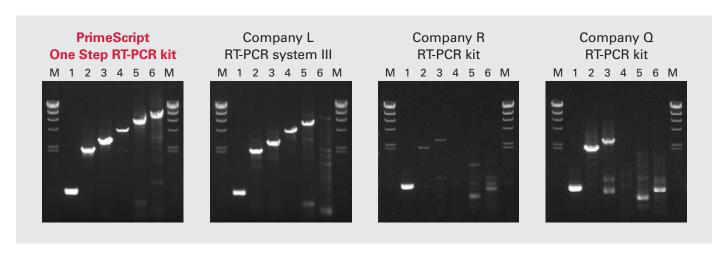
Comparison of Takara Bio one-step kit with competitor kits for long amplification. 1 μg of total human RNA was used as a template for cDNA synthesis. Each RT-PCR was performed according to the supplier's recommended conditions. Lane 1 is *TFR*, 0.5 kb. Lane 2 is *CCND2*, 2.1 kb. Lane 3 is *CCND2*, 2.8 kb. Lane 4 is *TFR* 4.4 kb. Lane 5 is Dystrophin, 6 kb. Lane 6 is Dystrophin, 8 kb. M is a control which contained a λ-HindIII digest.
